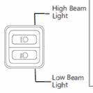
Remarks: To signal overtaking, the rider may press and hold the Pass button to enable the High Beam Light and Low Beam Light Interchange Mode. Release the Pass button to return to the Low Beam Light.
